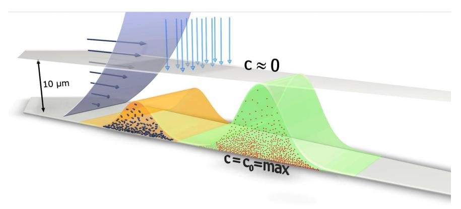
Separation based on diffusion against a cross-flow in a laminar flow stream
