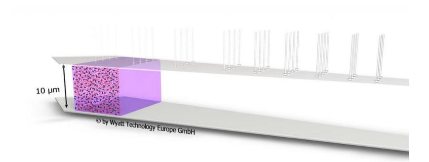
• Sample injected – by interaction with the cross-flow it is concentrated against the porous bottom wall
