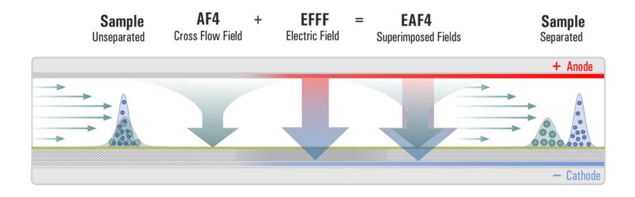
• EAF4 uses both force fields to generate a separation plus measurement of electrophoretic mobility
