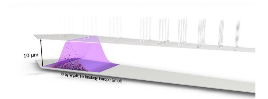
• The electrical field is added after focusing has taken place
