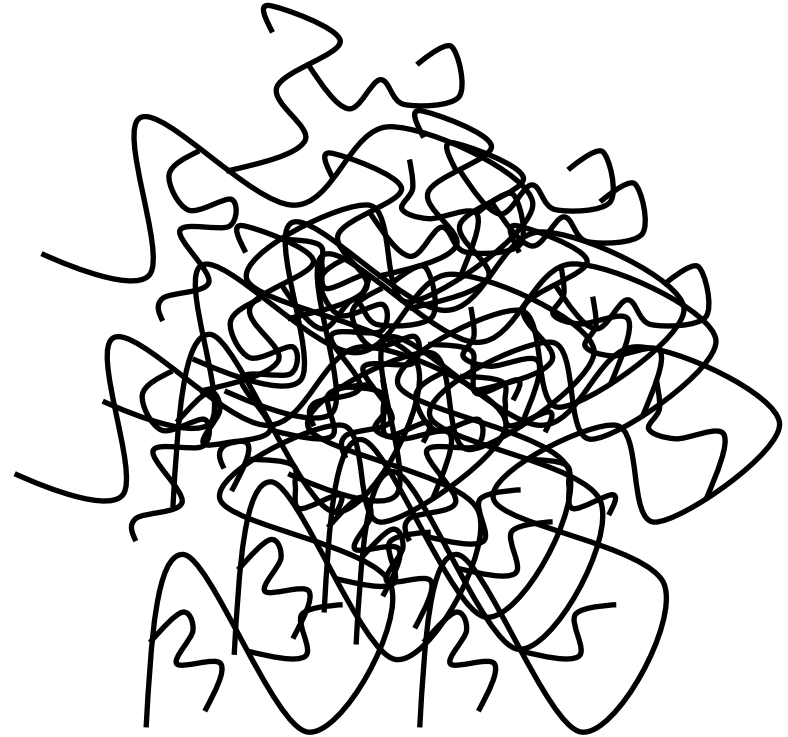
Crosslinked polymer (Insoluble, makroscopic gel, micro- or nano-gels)
