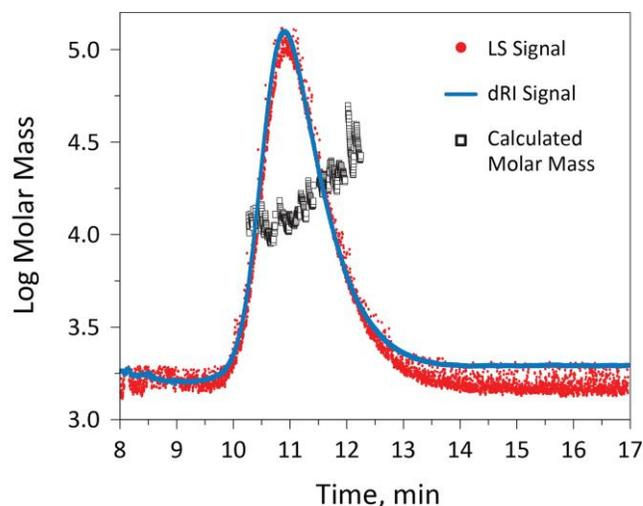
Fig. 9 AF4 separation of a lignosulfonate sample using a polyether sulfonate membrane. Molar masses are measured with a HELEOS MALS detector at 785 nm with fluorescence-blocking filters. As this sample has less fluorescence compared to lignin, correct values can be calculated.
