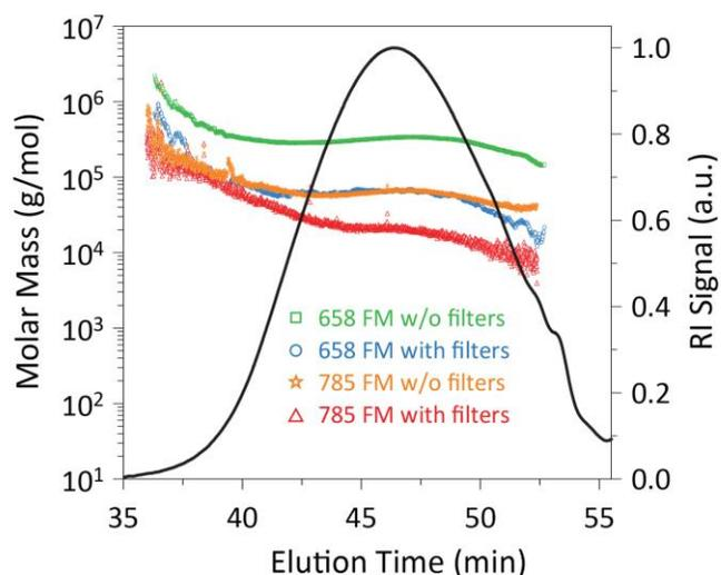
Figure 4. Comparison of calculated molar mass using different configurations of the MALS instrument. Two different laser wavelengths with and without fluorescence-blocking filters have been applied. At the infrared wavelength of 785 nm fluorescence is reduced compared to the 685 (red) wavelength. But even then, filters are necessary to minimize the effect of light not coming from scattering. (Figure adapted from Ref. 1)
