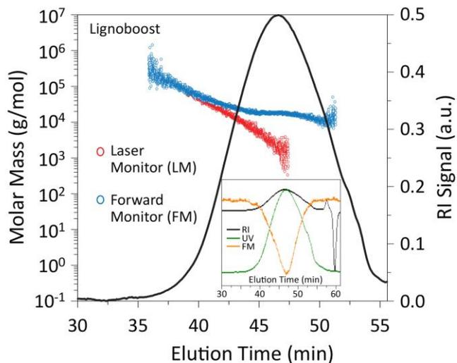
Figure 3. Effect of using the laser monitor (LM) or the forward monitor (FM) to calculate the molar mass of a strongly absorbing lignin sample. Using the LM which is the uncorrected laser intensity leads to an underestimation of the molar mass. The insert shows the forward monitor reading in an overlay with the RI trace. (Figure adapted from Ref. 1)
