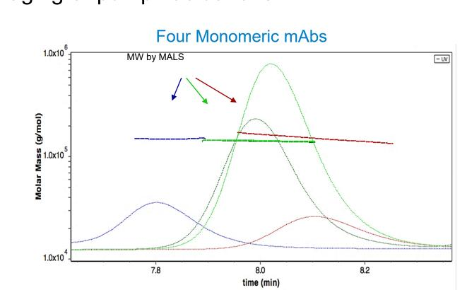
SEC-MALS: Determines molar masses independently of elution time, and does not require calibration against reference molecules. Hence MALS correctly characterizes:
